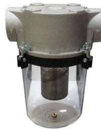
Liquid separators protect the pump from liquids in the air stream. A 50 mesh stainless steel screen traps large particulates. Float ball blocks vacuum when bucket is full. Includes bottom 1/2” drain.
