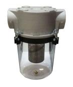
Liquid separators protect the pump from liquids in the air stream. A 50 mesh stainless steel screen traps large particulates. Inside the screen is a float ball that blocks vacuum flow when full. The clear collection bucket is quipped with a 3/4" drain.
