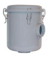
Standard compact filters are fitted with paper elements. They are easily removed by lifting the stainless steel torsion clips. Inlet and outlet connections are FPT.
