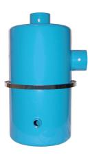
Combination liquid separator/vacuum filters are available with up to 6" connections. They are quipped with polyester elements that are 99%+ efficient to 5 microns. Constructed of carbon steel with epoxy coating.
