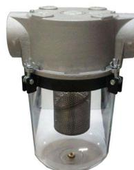
*Liquid knock out separator includes a stainless steel screen, internal float ball, and clear bucket with bottom drain.*
